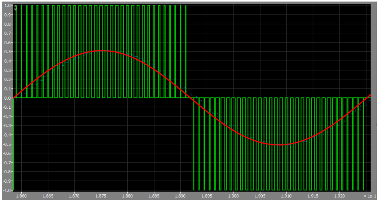
FIGURE 5 - THREE-LEVEL PWM SWITCHING; GREEN: PWM SIGNAL; RED: REFERENCE SINE SIGNAL
