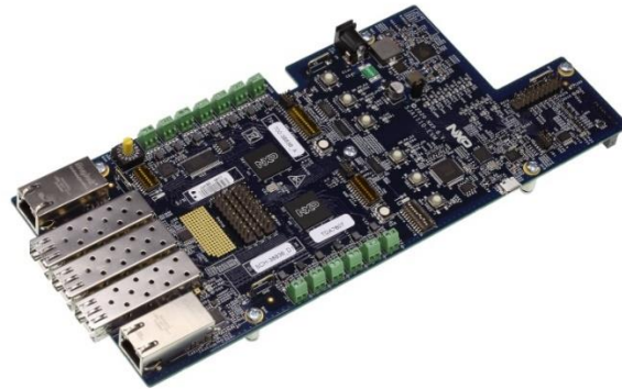
FIGURE 10: SJA1110 - EVM EVALUATION BOARD BY NXP
