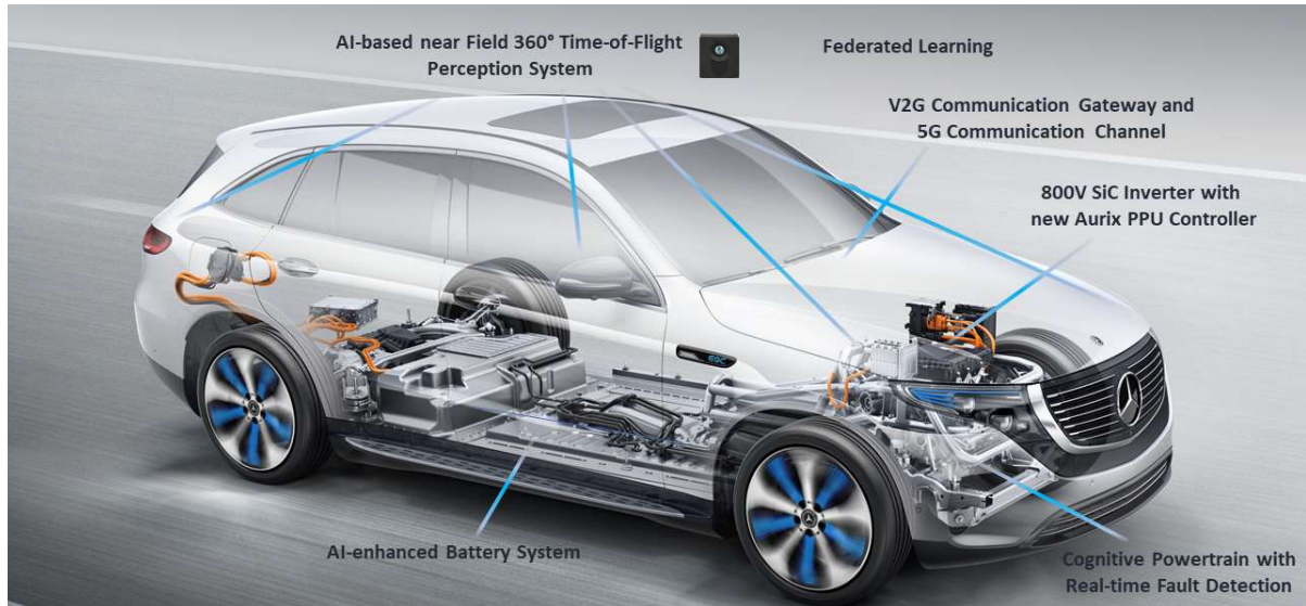
Figure 4. EV5.0 vehicle with real-time AI-based fault detection, analysis and mitigation
